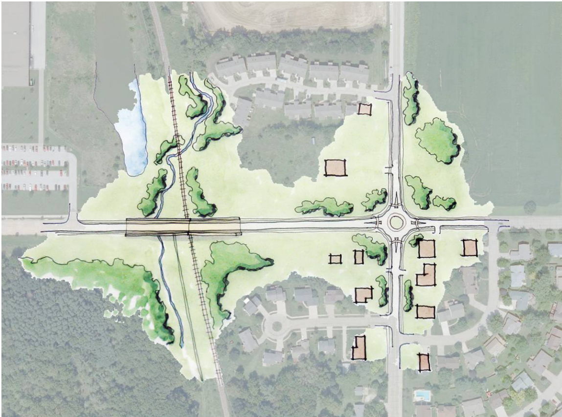
Proposed creek and railroad crossing on 46th Street, with roundabout at Eastern Avenue.
