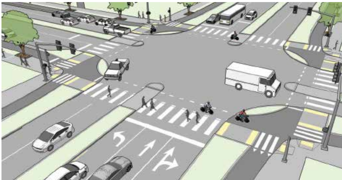
Figure 6.6: Intersection Concepts, Protected Intersection
