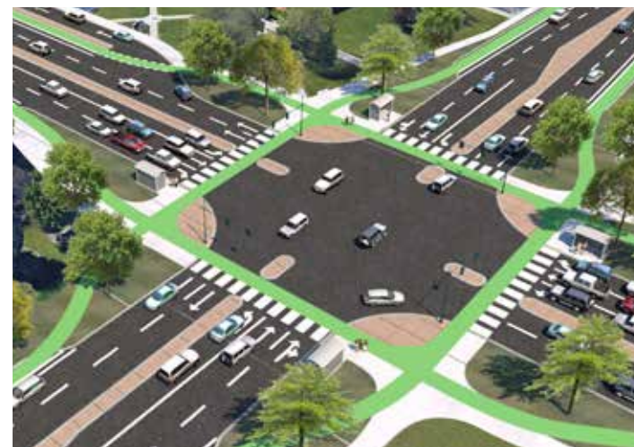
Top: Protected intersection in Salt Lake City. Above: Concept for an arterial crossing with bike lanes and paths in Wauwatosa, WI
